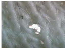
Holes cause by the needle (fibre melting)
